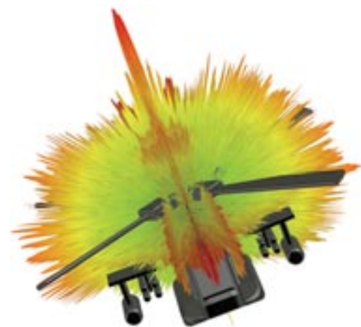
RCS & Surface Current Simulation of a Helicopter
