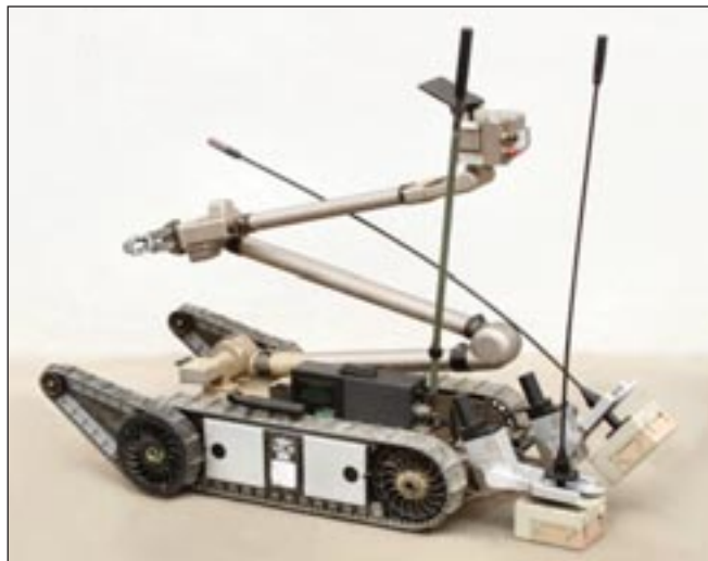
Figure 3. Fourth-generation ADCR system on an iRobot® PackBot®.
