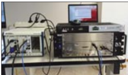
Hardware used to implement the Radar Target Simulator.
