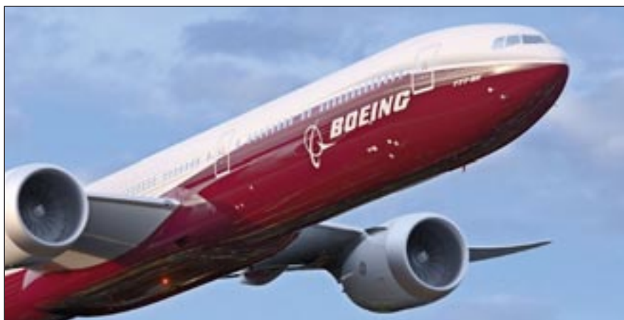
The new 777X will build on the 777 and will include new engines, an all-new composite wing and will leverage technologies from the 787 Dreamliner.
