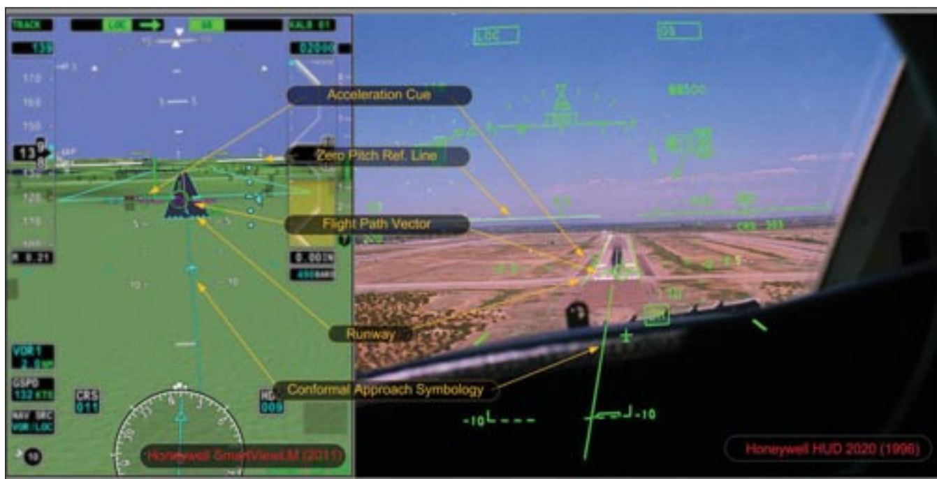
Figure 2. The integration between the Honeywell SVLM with FPV and runway approach symbology created in 2011 (left) based on Honeywell HUD2020 (right) created in 1996 providing the same functionality is shown above. LEFT: This screen capture is of an SVLM prototype installed in the company's Gulfstream 450. The approach shown was an ILS to runway 01 at Albany International Airport New York (KALB). RIGHT: This photograph was taken through the HUD combiner of the prototype HUD2020 installed in a Cessna Citation III. This approach was an ILS to runway 30C at Williams Gateway Airport, Phoenix Arizona (KIWA).
