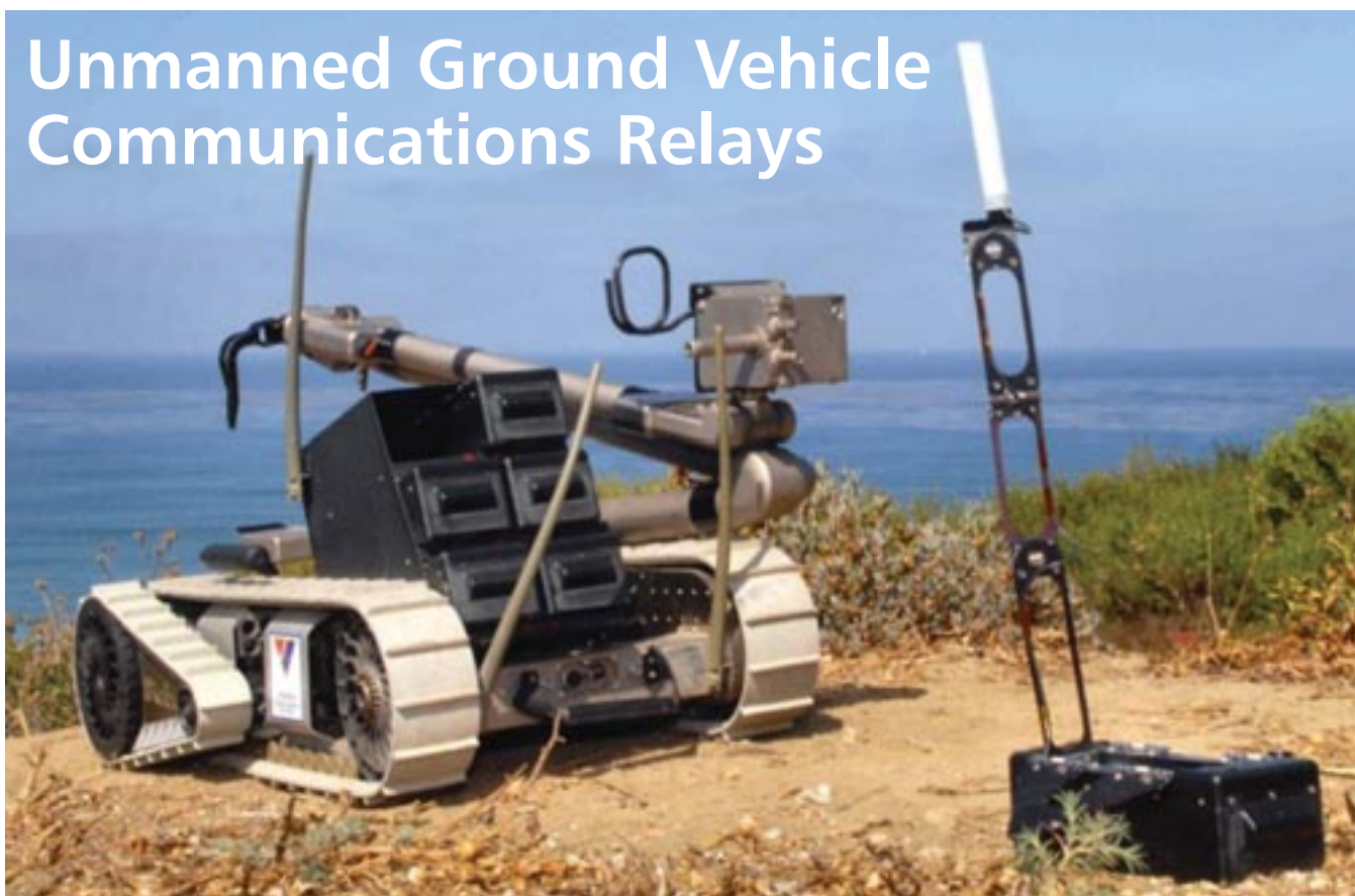
Figure 1. First-generation ADCR system on an iRobot® PackBot®.
