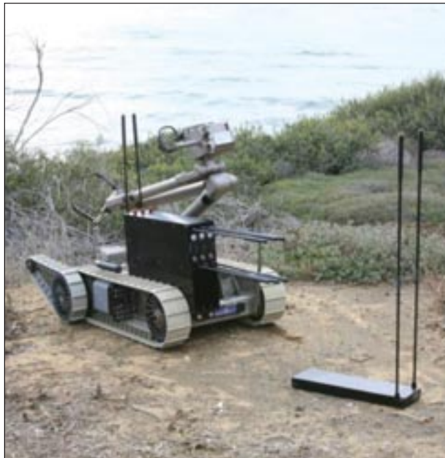
Figure 2. Second-generation ADCR system on an iRobot® PackBot®.
